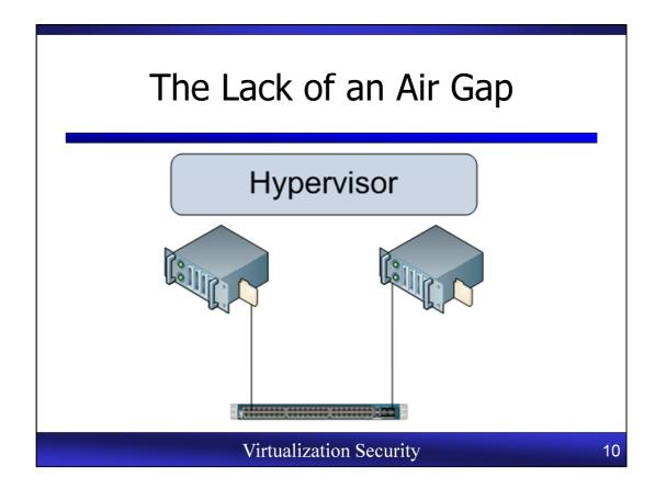
In a legacy network, some semblance of an air gap exists between operating systems. For example two systems connected to the same Ethernet network can only communicate with each other via the Ethernet network. If that network is disconnected or firewalled, the systems will be unable to communicate with each other.
