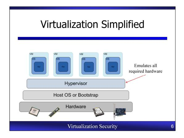
The above diagram graphically represents the layout of a virtualized platform. The hypervisor abstracts the VMs from the actual hardware by emulating these components. This can create a potential security bridge between the VMs, which we will discuss in greater detail later.
