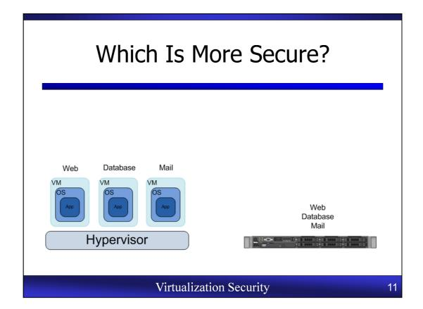
Consider the two deployments shown in the above slide. The system on the right represents how we have historically deployed servers. While we would ideally like to isolate each service to its own server, the reality is hardware availability and cost typically force us to combine multiple services onto the same system. This means that if any one of these services are compromised, the other services will quickly fall as well.
